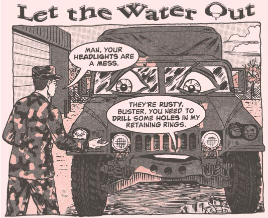
If rust is attacking the headlight retaining rings on your HMMWVs (or any other wheeled vehicle, for that matter), take a drill to the rings.
